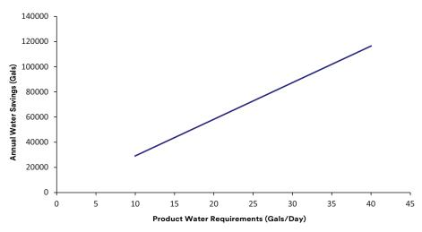
The SGLP-CL System from 3M results in considerable cost savings in both water utility and water sewage as compared to traditional RO systems. In fact, a restaurant can save nearly 400 gallons of water for every 50 gallons of water used!
